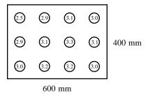
The duct cross-sectional area is:  $0.600 \times 0.400 = 0.240$  meters<sup>2</sup>, therefore, the volume flow rate is  $0.240 \times 3.025 = 0.726$  cubic meters per second.
