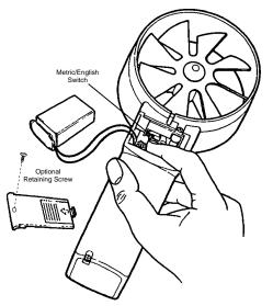
Figure 1: Battery compartment detail
