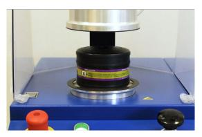
Respiratory filter cartridge placed into the Automated Filter Tester 8130A
