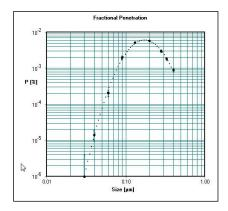
MPPS and fractional penetration results measured with Automated Filter Tester 3160
