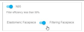
If/when your organization uses the OSHA Fast fit testing protocols, having this field configured correctly will help guide fit test operators to select the correct version of the protocol to use for the respirator being fit tested, "OSHA FAST-Filtering Face" for a "Filtering Facepiece" or "OSHA FAST-Full/HALF FACE" for an "Elastomeric Facepiece":
