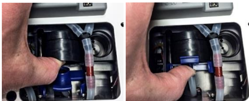
Figure 35: Snap cassette securely into inlet port
