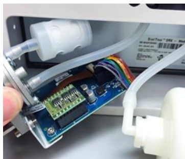
Figure 28: Pull pump from enclosure and detach tubing, muffler, and cable
