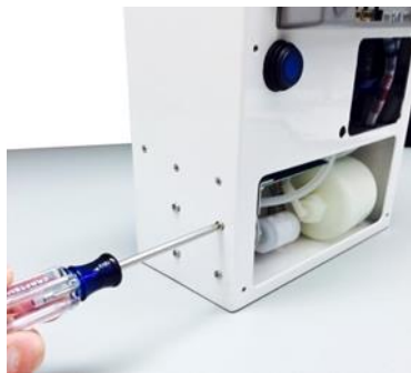
Figure 27: Remove screws from left side panel
