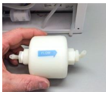
Figure 21: Disconnect and remove old sheath air filter
