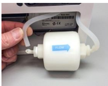
Figure 21: Disconnect and remove old sheath air filter
