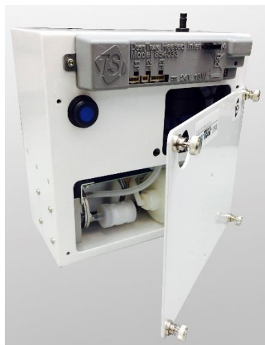
Figure 20: Open instrument service panel
