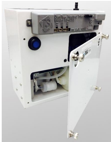
Figure 26: Open instrument service panel
