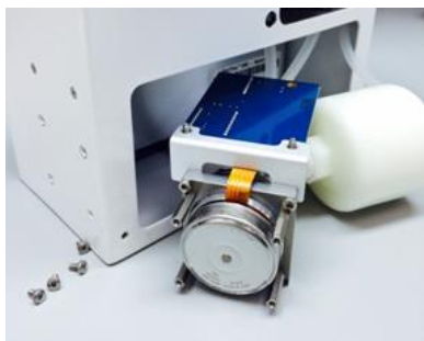
Figure 28: Pull pump from enclosure and detach tubing, muffler, and cable
