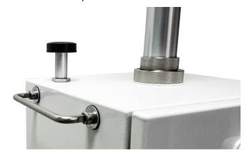
Install heat shield over the inlet and rest it on the handles.
