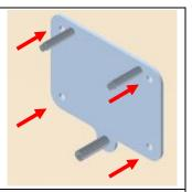
2. Attach the Meter Plate to the Meter using the three (3) supplied M3 screws.
