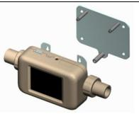
Use one (1) supplied #8 screw in the bottom frontfacing screw hole to secure the instrument.
