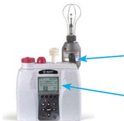
Connect AirProbe to the Back Housing
