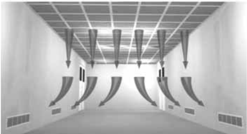
Figure 7 Unidirectional displacement of dirty air
