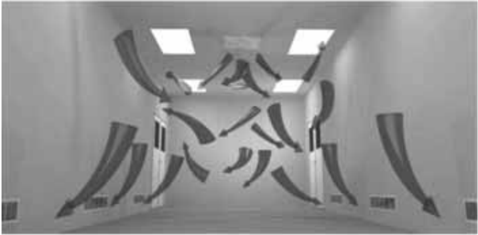
Figure 6 Turbulent dilution of dirty air
