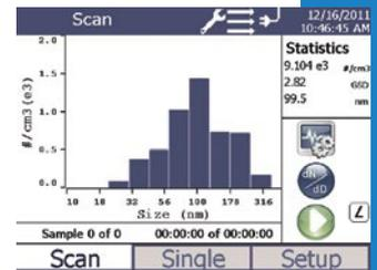
Screen shot of NanoScan SMPS during nanoparticle size distribution measurement
