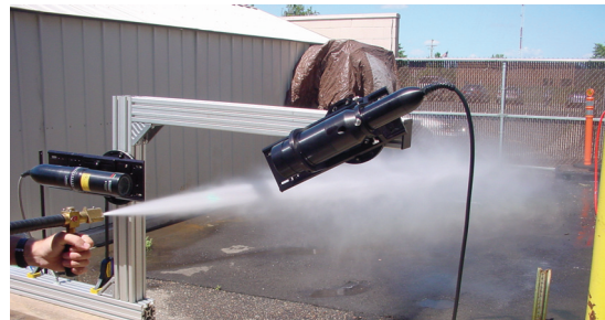
Figure 2: UHPS fire suppression spray (water) being measured by a TSI PDPA system
