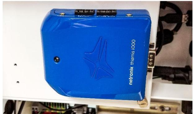
7. Connect the GSM and GPS antenna cables to the modem.
