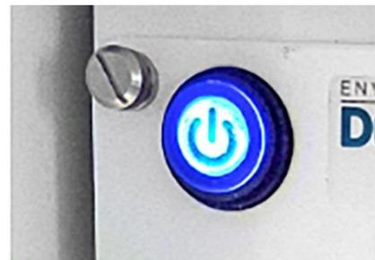
11. The LED on the modem will blink while the modem searches for a suitable network. If the LED stops blinking and is solid blue, a network has been found and proper communication with Environet™ should be possible. If the LED changes to solid yellow, the modem has not found a network. A power cycle may resolve the issue or the unit may need to be moved to a different location where signal strength is improved.
