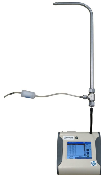
Probe and Coupler Connected to OPS
