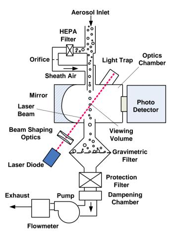
constant which is determined from the ratio of a known mass concentration of the test aerosol to the voltage response of the DustTrak<sup>™</sup> II Aerosol Monitor. Typically, the test aerosol is Arizona Test Dust (or ISO 12103-1, A1 test Dust).
