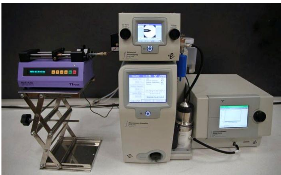
Figure 1: Model 3482 Electro spray Aerosol Generator (EAG) used with syringe pump and Model 3938 Scanning Mobility Particle Sizer™ (SMPS™) Spectrometer
