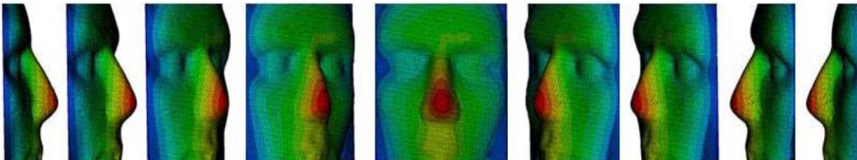
Figure 2: A single recovered 3-D image of the headform shown from nine different points of view.
