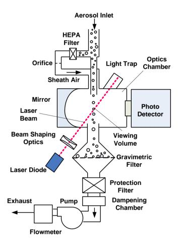
constant which is determined from the ratio of a known mass concentration of the test aerosol to the voltage response of the DUSTTRAK II Aerosol Monitor. Typically, the test aerosol is Arizona Test Dust (or ISO 12103-1, A1 test Dust).
