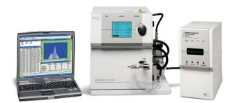
charge matrix for radioactive <sup>85</sup>Kr-Neutralizer and Soft-x-ray based neutralizers. This Application Note describes the steps how to use the charge matrix for soft-x-ray neutralizer as an alternative to the default Kr-neutralizer charge matrix in older SMPS systems (Model 3936, based on Electrostatic Classifier 3080 or 3071) running with Aerosol Instrument Manager software (version 9).
