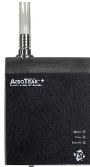
Connecting Sample Tubing to Remote Active Air Sampler
