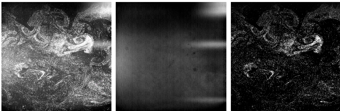
Fig. 4. Benefit of image background subtraction. The images shown are the original image (left), background image (center), and background-subtracted image (right).
