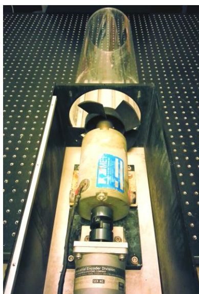
Fig. 1. Photograph of the fan and duct used in the current experiment. The cover has been removed from the motor housing for clarity. The cover was in place for the experiments.
