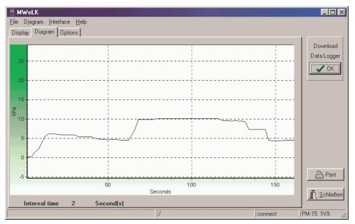
The loaded values are indicated as line graphics. As the software always indicates the stored values with the maximum scaling it is recommended to zoom, enabling specific extracts to be enlarged.
