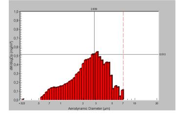
The aerodynamic size distribution of the suspension pMDI again is a non-Gaussian one that indicates two modes. The 3D-plot reveals this even more clearly: one mode is of a very narrow, submicrometer aerodynamic size with a wide light scattering range, while the other mode ranges from 1 to ~6 µm in aerodynamic size but only a small scatter around an intensity of about 10.
