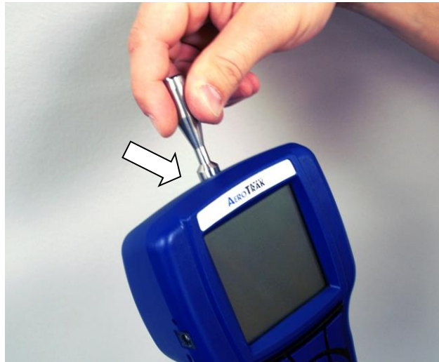
Installing an Isokinetic Inlet
