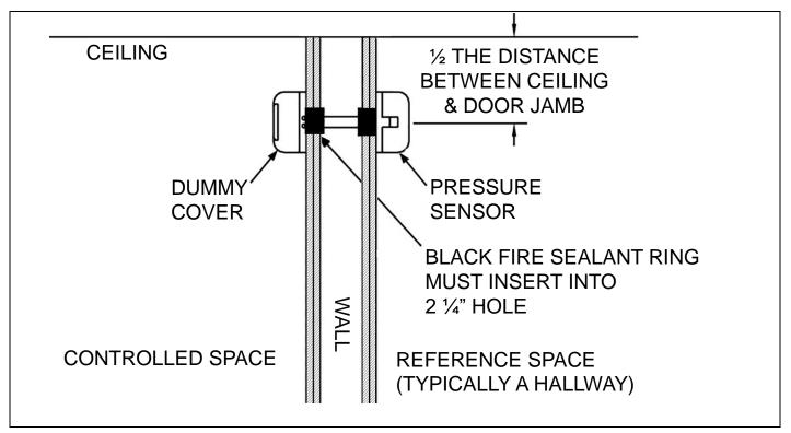
Figure 3: Cutaway View of Mounted Pressure Sensor
