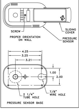
Figure 2: Pressure Sensor Orientation and Mounting Template
