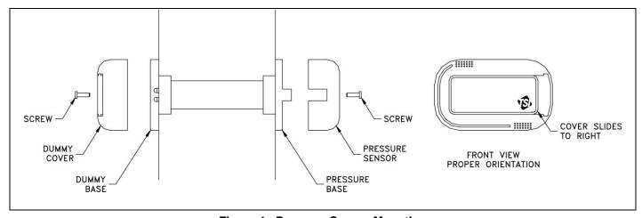
Figure 4: Pressure Sensor Mounting
