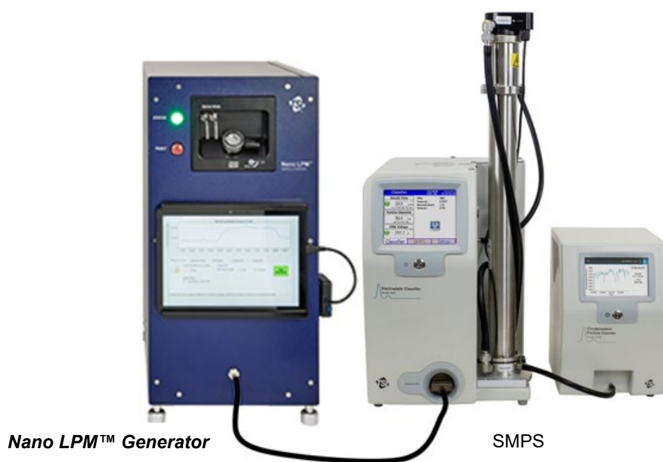
Figure 2. Nano LPM™ Generator and SMPS system used for characterizing the PSD of CMP slurries.
