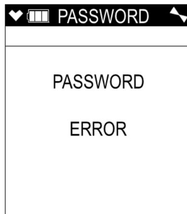
You must turn the unit off and reenter Maintenance Mode 2 using the correct password.
