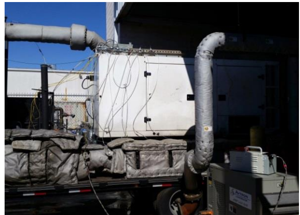
Figure 3: NPET measuring DPF condition of a John Deere 6068TF275 diesel engine stationary generator
