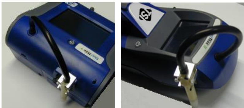
Figure 2-8: Installing Door-Oliver Cyclone
