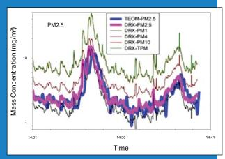
Comparison of Arizona Road Dust mass concentration measured by the DustTrak DRX and the TFOM with a PM2.5 impactor.
