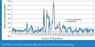
The PM2.5 24-hour average data from the DustTrak Environmental Monitor is shown to compare extremely well with the E-BAM (slope of 0.993 and R^2 of 0.99), as supported by the correlation plots above.
