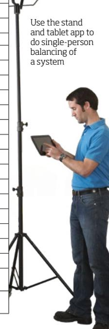
Use the stand and tablet app to do single-person balancing of a system
