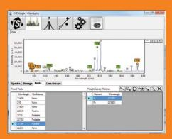
Automatically identify elements in OES spectrum or match entire spectra with library entries to identify materials.
