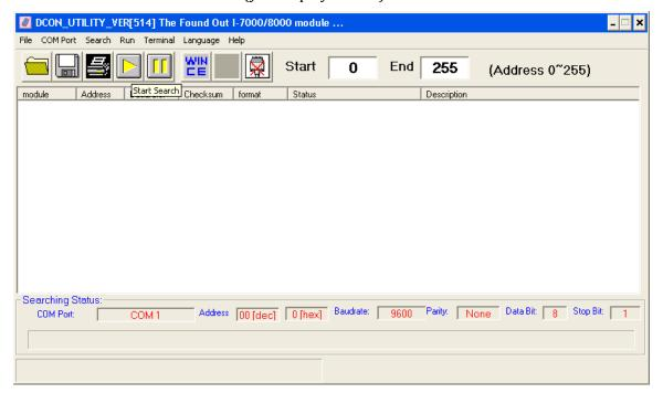
4. Application will start running search and all detected controllers on given serial port will display.
