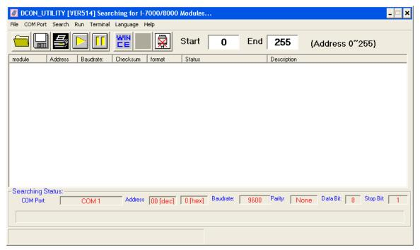
2. Under **COM Port** menu, select the communication port to which RS-485 converter is attached and select settings shown.
