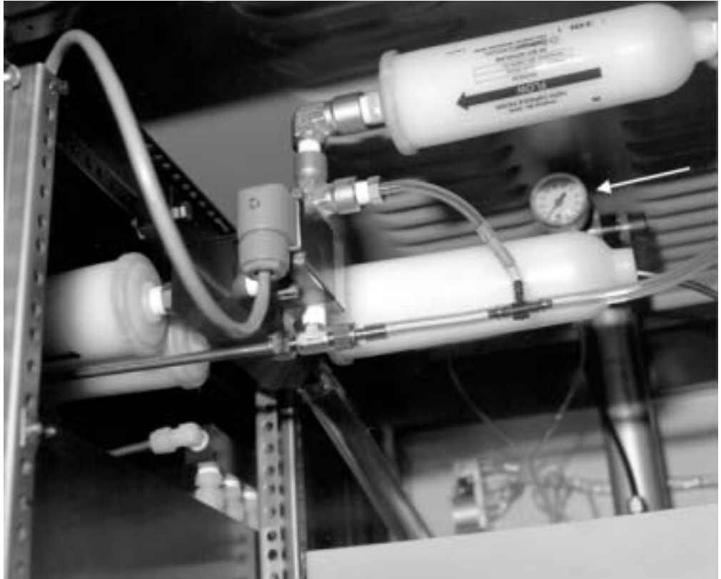
Figure 5-3 Filter Holder Pressure Regulator
