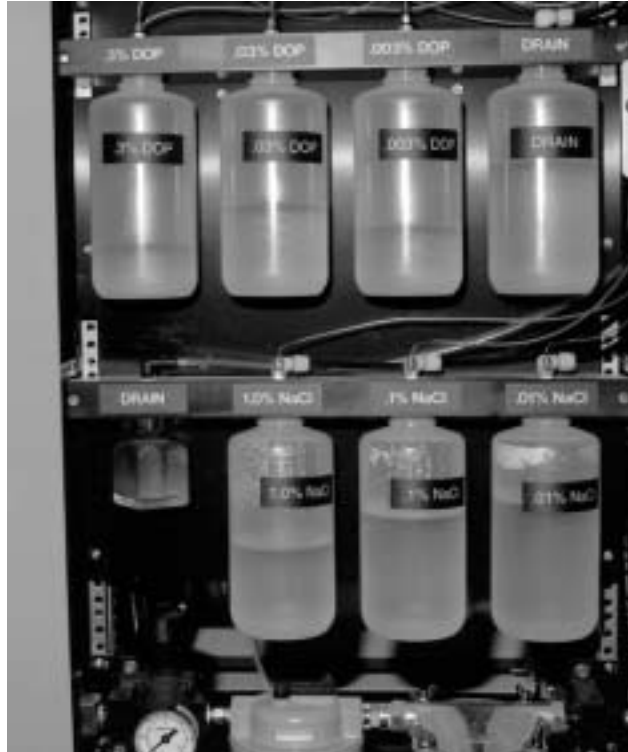
Figure 2-12 Aerosol Generator Bottles
