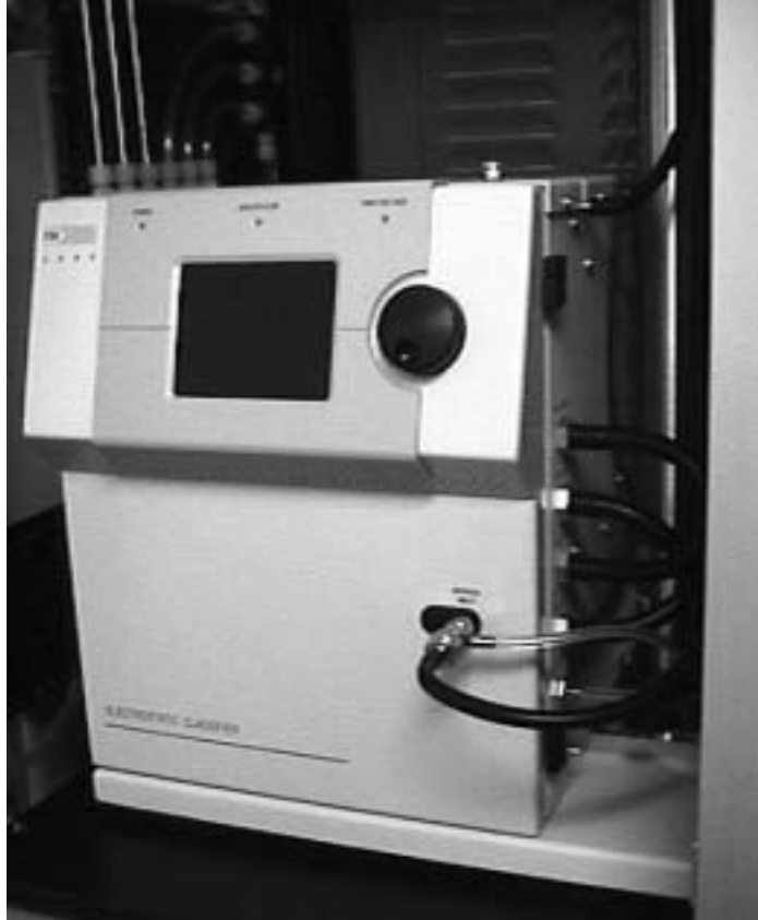
Figure 2-6 Electrostatic Classifier Installed
