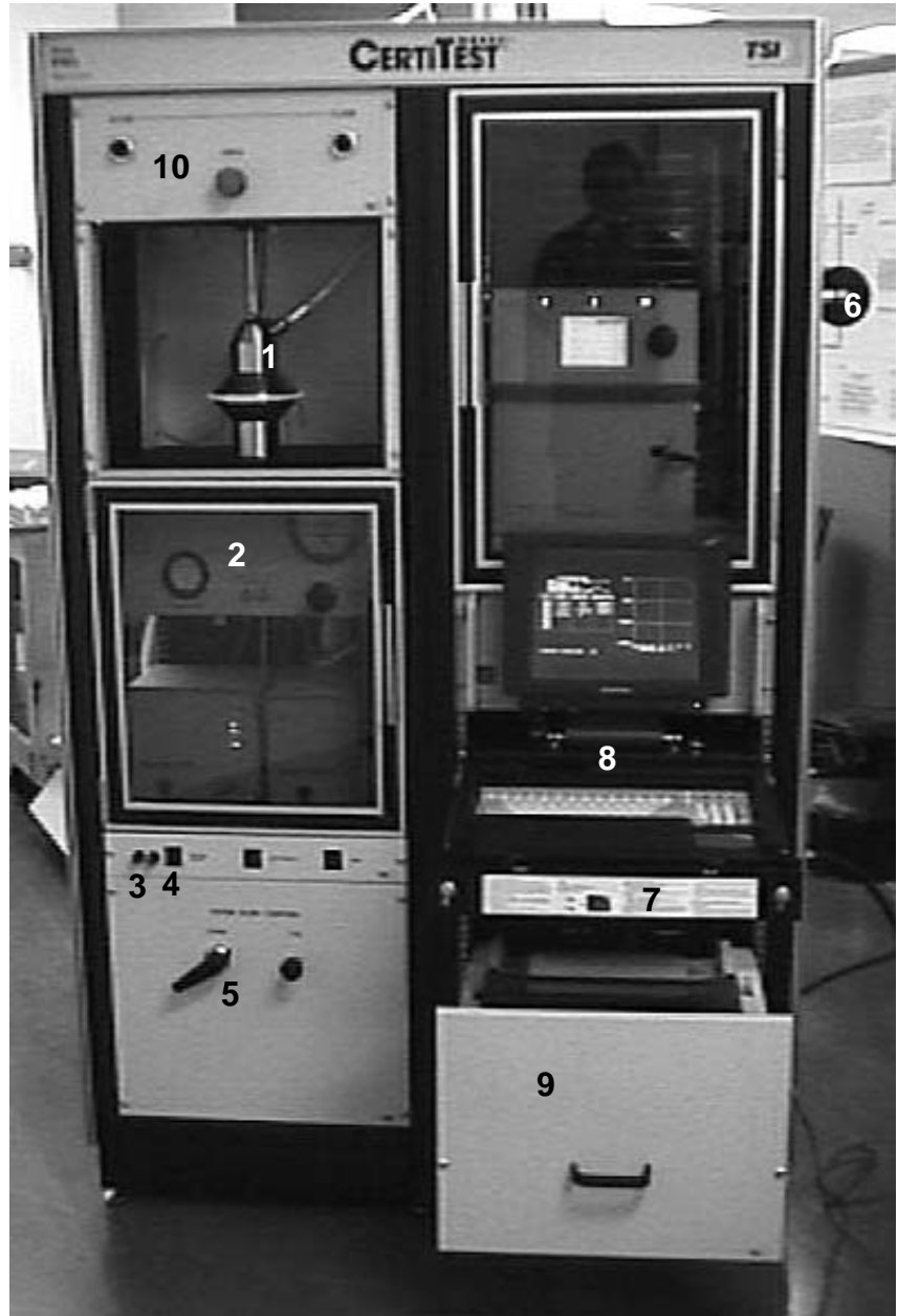
Figure 2-1 Front View of the Model 8160 Automated Filter Tester
