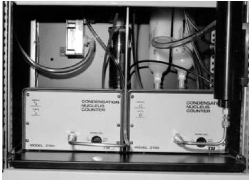
Figure 3-1 The Condensation Particle Counters (CPCs)
