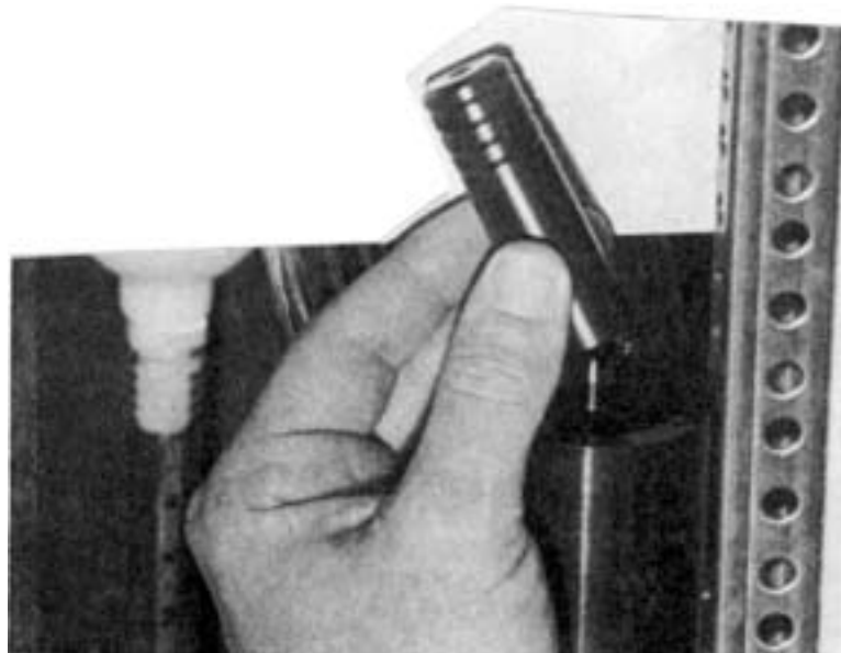
Figure 8-9 Use Insertion Tool to Press Diluter Tube in Place
