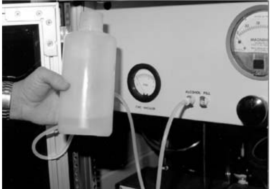
Figure 8-1 Filling the CPC with Butanol
