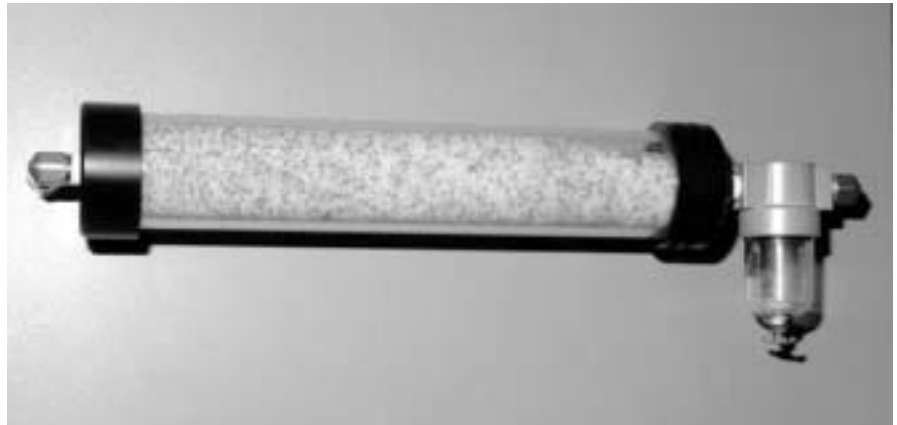
Figure 2-10 Aerosol Diffusion Dryer
