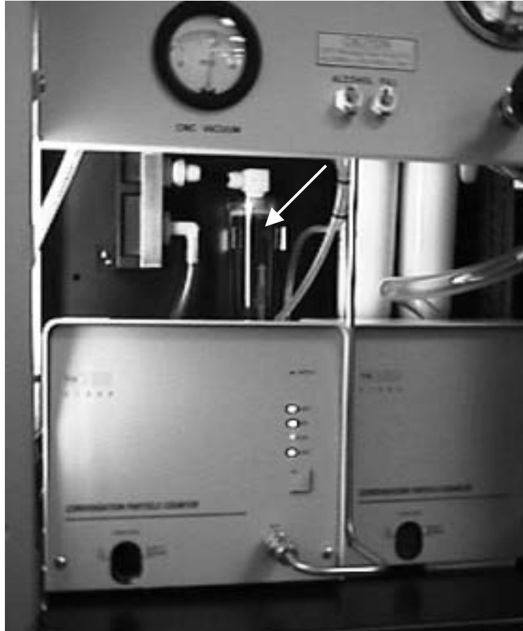
Figure 8-3 Replacing the CPC Carbon Filter
