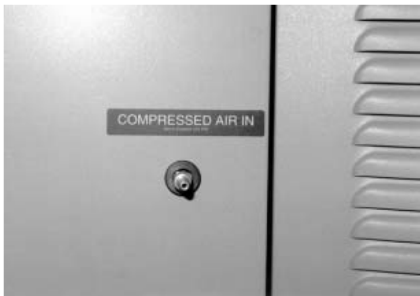
Figure 2-11 Compressed Air Inlet
