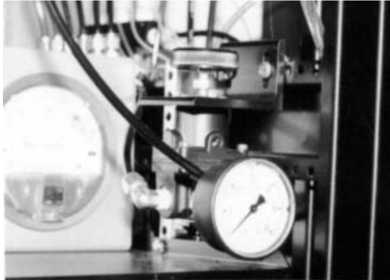
Figure 5-2 The Aerosol Generator Pressure Regulator
