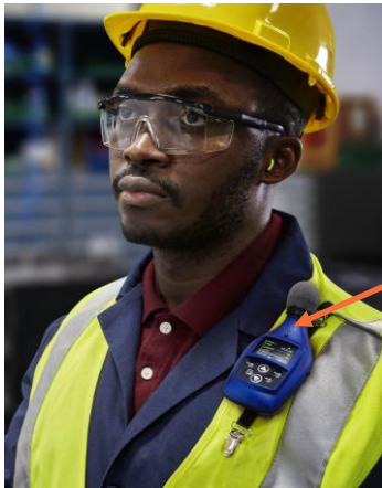
Figure 4-2: Attaching the Edge on your shoulder
