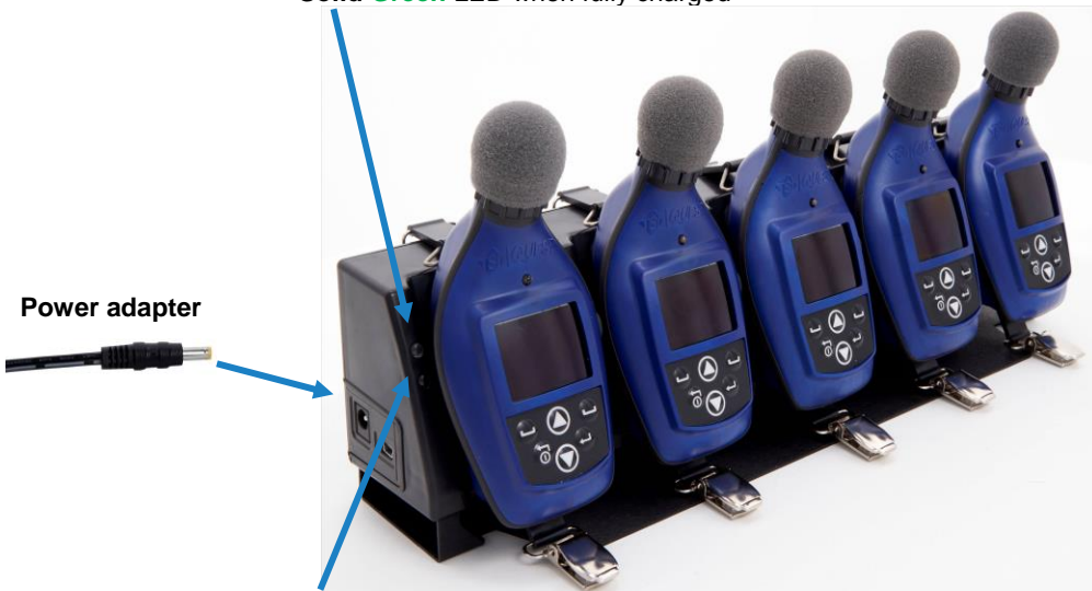
Figure 2-7: Docking the Edge on the EdgeConnect
