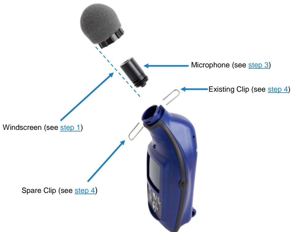
Figure 6-1: Microphone and windscreen assembly
