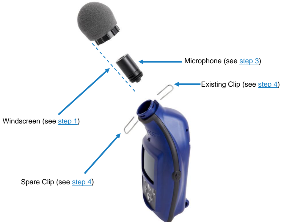
Figure 6-1: Microphone and windscreen assembly
