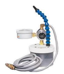
jet located in the jet-nozzle assembly. The jet creates an area of low pressure near the orifice which, in turn, causes the liquid in the reservoir to be sucked up into the orifice. The liquid is then broken into tiny liquid droplets and the compressed air carries the droplets through the outlet tube.
