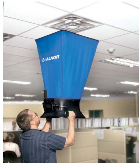
EBT731 Balometer® hood measuring a supply diffuser
