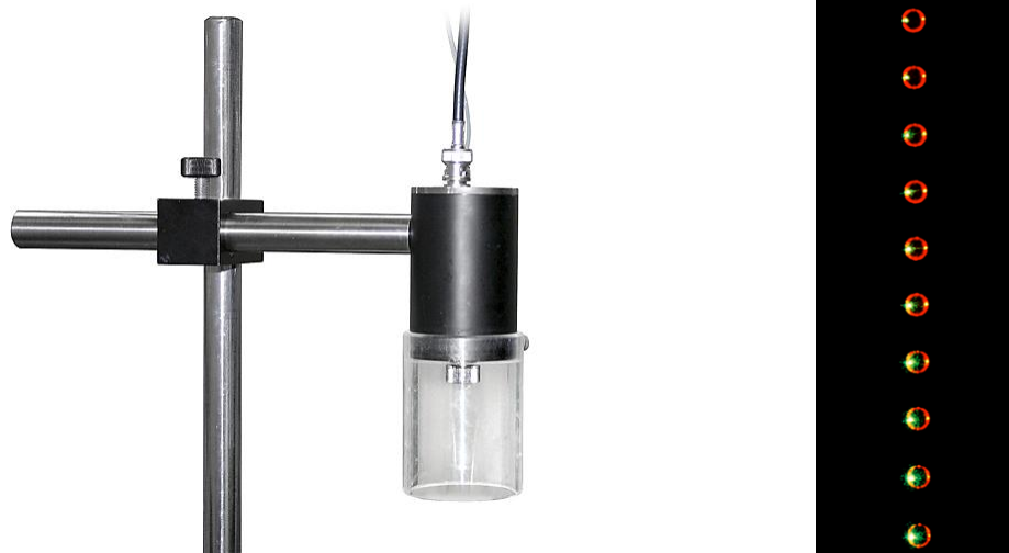
Figure 1. MDG-100 Vibrating orifice head (left), and resultant droplet stream (right).
