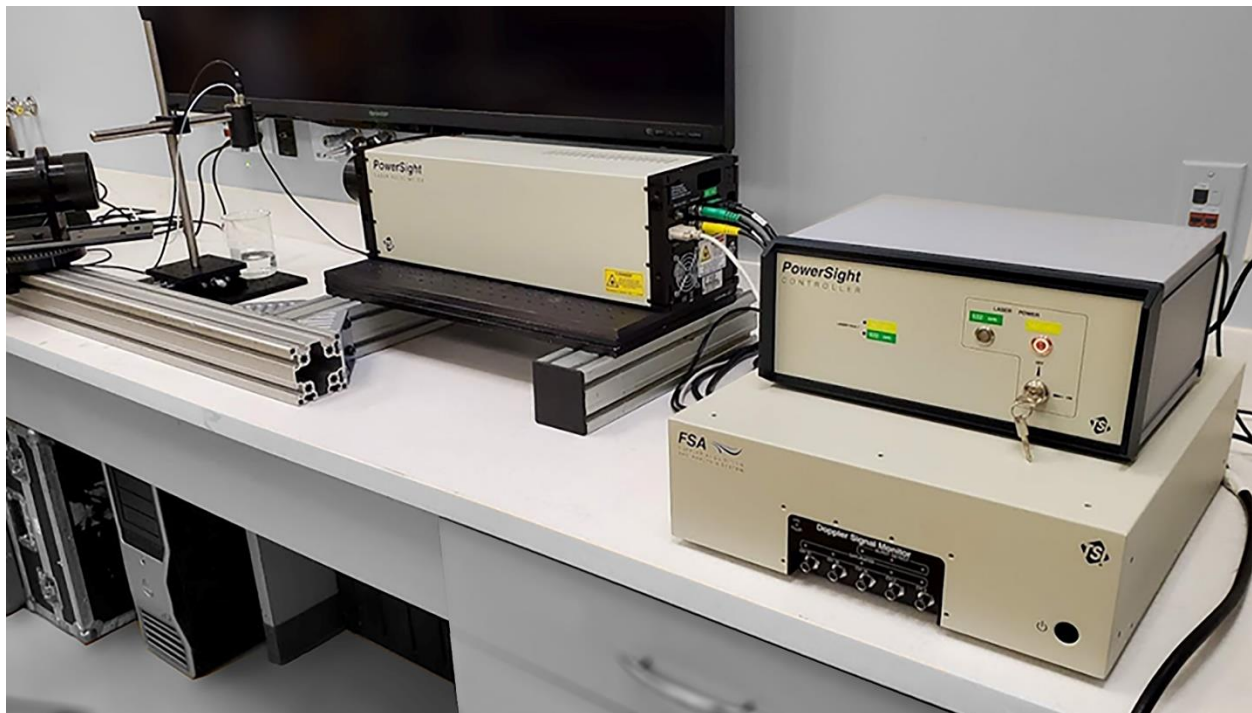
Figure 2. PDPA system aligned for taking size and velocity data on an MDG-100.
