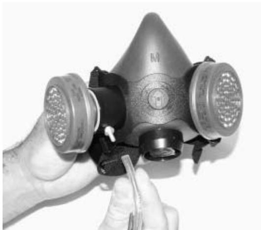
3. Press the TEST START/STOP key to start the fit test and instruct the individual to begin the first exercise. A single audible "beep" signals the end of an exercise and the immediate beginning of the next exercise. There is no pause between exercises. During an exercise, the fit factor from the
