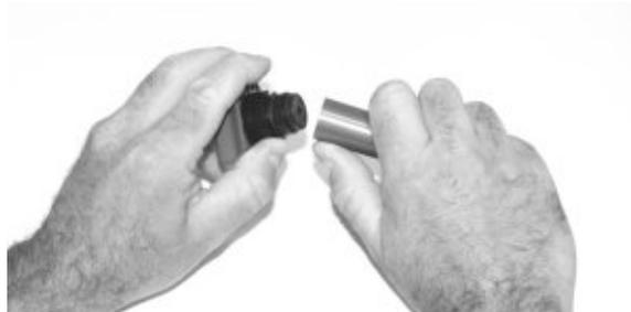
After separating the two halves, push the Alcohol Wick and screen out of the Wick Retainer Cap from the opposite end with the Wick Removal Tool (wood dowel) provided with each new alcohol wick. Do **not** use a pencil point because bits of lead could break off. Allow the small, circular, fine-mesh screen to fall out on the table.
