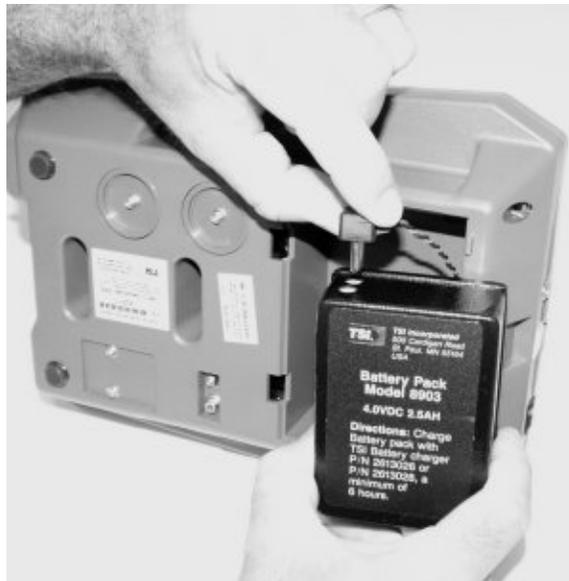
3. Place the battery pack into the battery compartment in the orientation shown. Tuck the wires in so that they do not interfere with closing the battery cover. Make sure the wires are not allowed to be underneath the battery.
