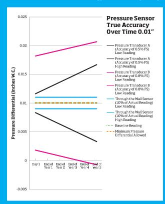
The best-in-class stability of TSI's unique room pressure sensor lets you avoid time-consuming sensor recalibrations.
