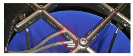
3. The short tubing ends can be inserted into the pole support bracket to keep them out of the way.
