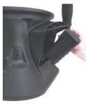
2. Disconnect the short tubing from the ports on the flow manifold.
