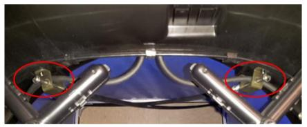
4. Use the two 8 ft. (2.4 m) sections of tubing included with the instrument to connect meter directly to flow manifold
