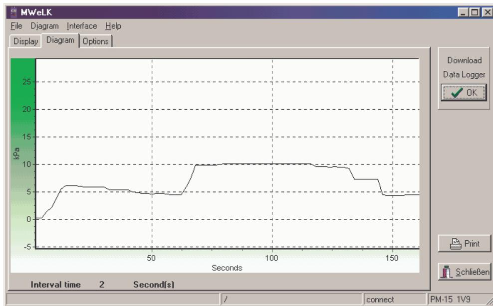
The loaded values are indicated as line graphics. As the software always indicates the stored values with the maximum scaling it is recommended to zoom, enabling specific extracts to be enlarged.
