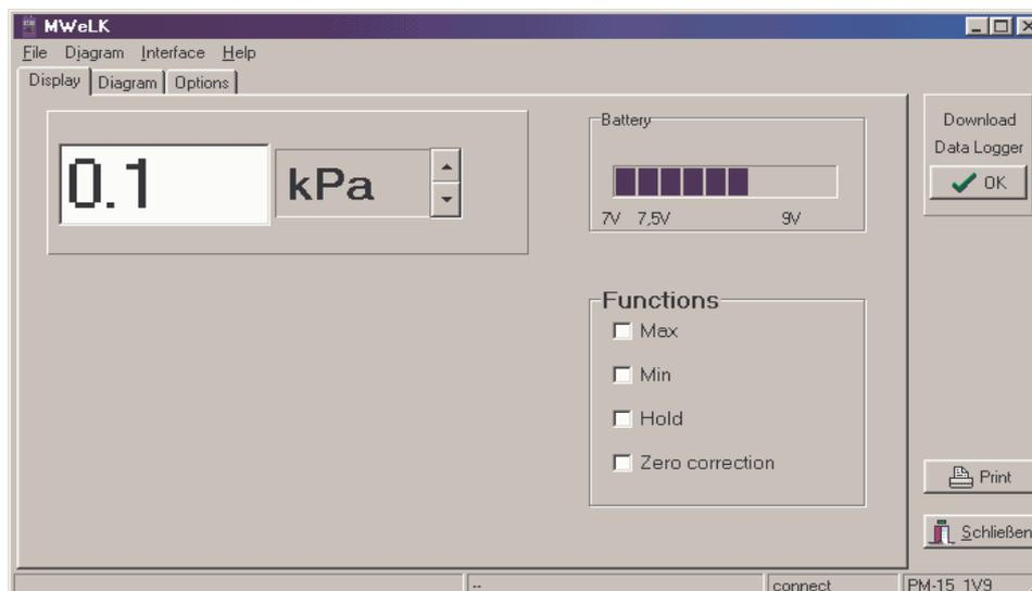
With the arrow keys next to the unit indicator, other units can be selected. The functions Min, Max, Hold and Zero correction can be activated or deactivated by mouse click. The current battery voltage is indicated by a bar graph.
