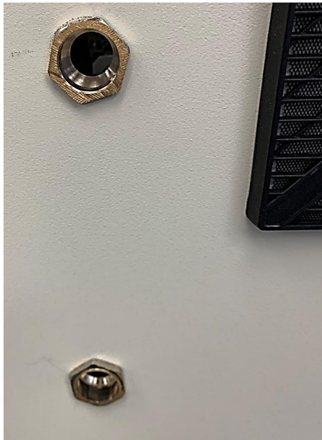
Figure 6. The metal grommets in the PTT front cover panel.
