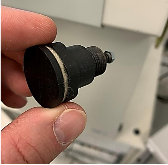
Figure 2. The factory-installed vacuum pump muffler removed.
