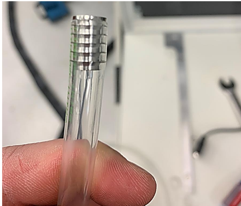
Figure 4. A piece of the 3/8 in. OD polyurethane tubing with the tubing inserts installed.
