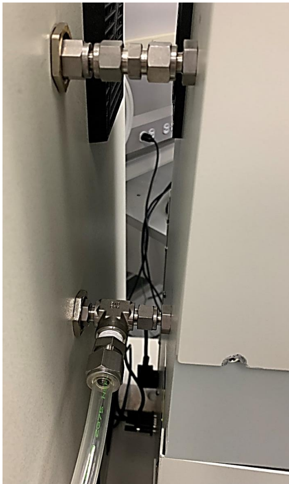
Figure 10. The exhaust adapter fittings installed and tightened.
