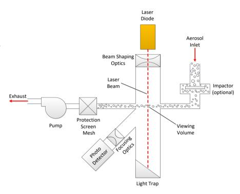
constant to yield factory calibrated mass concentration. The internal calibration constant is determined from the ratio of the voltage response of the SidePak™ AM520/AM520i monitor to the known mass concentration of the calibration test aerosol (A1 Test Dust).
