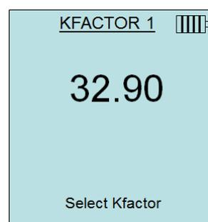
Make adjustments to the indicated value with the ▲ or ▼ keys and press ← to accept, or enter the **Select Duct** or Select **Kfactor** menu to choose a different pre-programmed flow value or dimension depending on instrument model:
