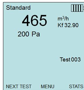
When measuring **Flow** as the **Primary** measurement, the parameters can be quickly changed by pressing the ▲ or ▼ key while on the main measurement screen:
