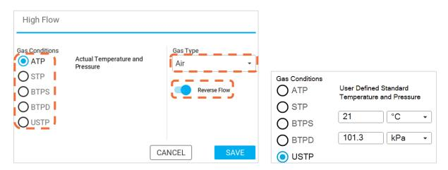
To specify your own temperature and pressure values and apply those conditions to gas flow measurements, select the **USTP** gas condition option (shown above right).
