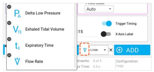
To change the units of measurement for a parameter, press on the currently selected units to access a drop-down list of available alternatives (see below right). Refer to the table <a href="Available Units of Measurement">Available Units of Measurement</a> to see all the available units for each measurement.
