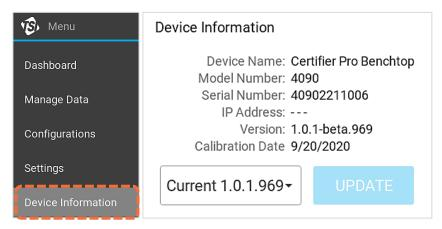
The Version field lists the firmware version currently implemented for the Certifier™ Pro Flow Analyzer. The Calibration Date field is set by TSI<sup>®</sup> during calibration service as part of the sensor adjustment process.
