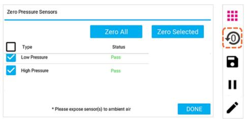
After zeroing, a status is displayed for each pressure sensor to indicate the result of the zero process. The pressure sensors can be zeroed more than once by you while in the **Zero Pressure Sensors** screen. Press the **DONE** button to return to the Certifier™ dashboard screen.
