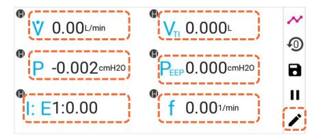
Press the **(+) ADD** tile to select an additional measurement, or press the measurement symbol of a currently selected measurement to change that measurement parameter.
