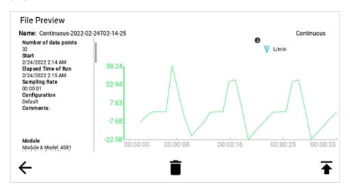
Saved files can also be deleted or exported from within the **File Preview** screen using the buttons on the bottom of the screen. Press the left arrow icon to return to the **Manage Data** screen. Press the garbage can icon to delete the currently previewed file, press the up arrow icon to export the currently previewed file.
