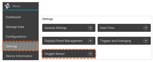
3. In the **Oxygen Sensor** screen, the Certifier<sup>™</sup> Flow Analyzer will display any connected oxygen sensors. Press the **Calibrate** button and follow the on-screen directions to complete the calibration process.
