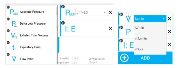
To reorder the selected measurements, press and hold a measurement tile to be able to drag it around the display. The other tiles will adjust on the screen as the tile is being dragged, release the tile once the desired position has been reached.
