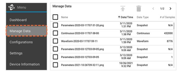
The **Manage Data** screen lists all the individual saved data files and screenshots available to the user. The **Data Type** column corresponds to the Certifier<sup>™</sup> logging options and files are labeled as either **Snapshot**, **Continuous**, **Waveform**, or **Graph**. The **# of Samples** column denotes the number of data points collected for each file and equals the sampling rate multiplied by the collection time.
