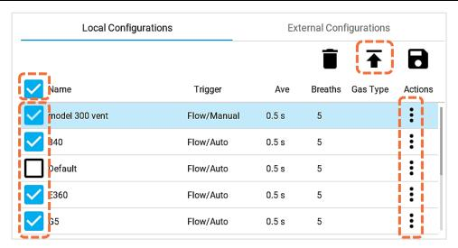
After configurations have been exported, you can navigate to the **External Configurations** tab to confirm that configuration files have successfully exported to the inserted USB drive. Exported configuration files can be attached in emails and imported into other Certifier™ Pro Model 4090 or Certifier™ Plus Model 4089 instruments.
