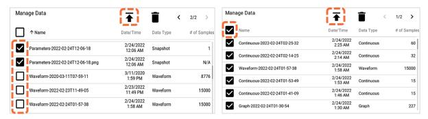
While actively exporting files, a loading icon will appear and the export progress is shown in the bottom screen bar. The Certifier™ Flow Analyzer will provide notification when the export has completed.
