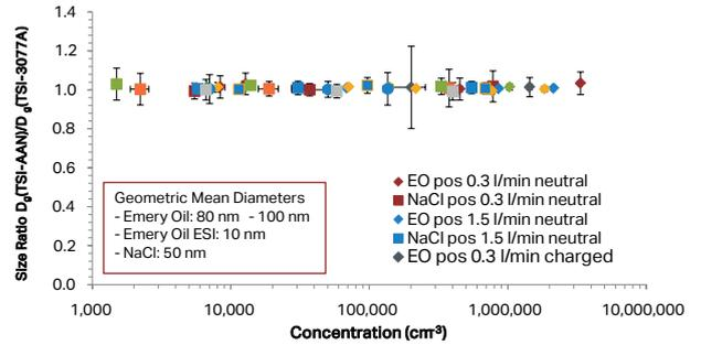
**Figure 1:** Ratio of the geometric mean diameter calculated from SMPS size distributions measured using a component system with a TSI Advanced Aerosol Neutralizer (AAN) versus a system with a TSI Aerosol Neutralizer 3077A.
