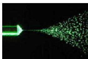
Liquid sample spraying from the capillary tip
