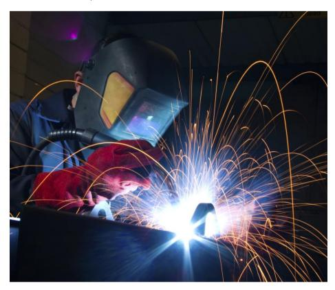
The invisible health risks are not as well understood. Welding generates ultrafine particles of smoke and fume, which can be inhaled by workers. If not properly controlled, compounds in welding fume, like manganese and hexavalent chrome, have been found to cause Parkinson's-like symptoms and cancer<sup>1</sup>.
