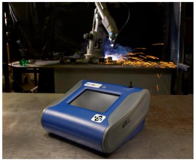
samples to a lab for analysis with results 10 days later, the DustTrak Aerosol Monitor provides aerosol mass concentration in real time, all day every day.
