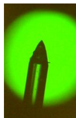
Cone-jet indicates flow
