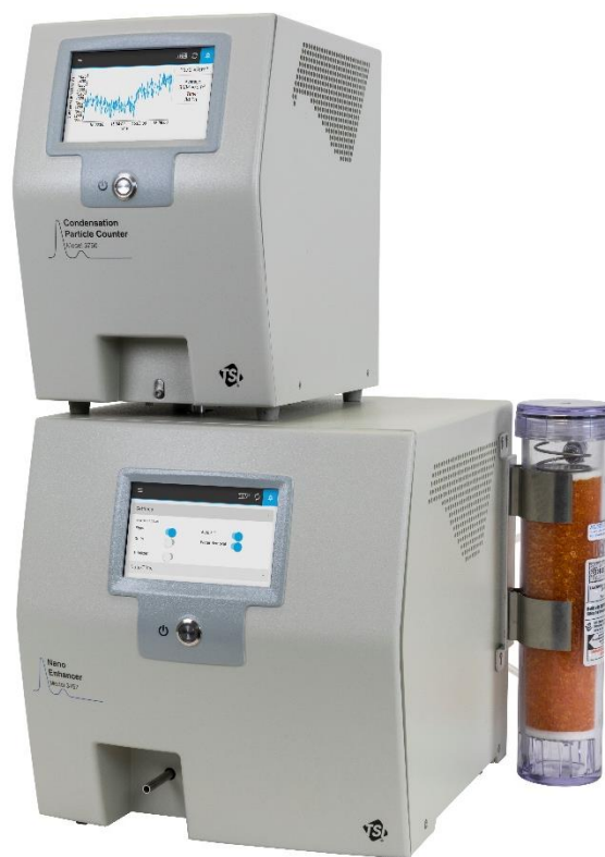
Figure 3: 1nm CPC system consisting of a Model 3757 Nano Enhancer coupled to a Model 3750 CPC
