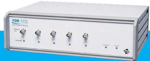
TSI's Photodetector Module (PDM) system combines an enhanced scattered light separation unit with high performance photodetectors for Phase Doppler Particle Analyzer (PDPA) and Laser Doppler Velocimeter (LDV) applications. The system is optimized for the best dynamic and operating size ranges, yet allows the freedom to adjust system parameters easily. System operation is controlled by TSI's FlowSizer™ Data Acquisition, Analysis and Display Software.
